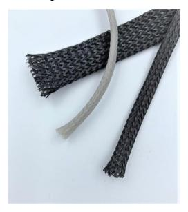
Polyester expandable sleeving is standard flame-retardant. It offers durable abrasion resistance in a wide range of industrial applications. The open weave construction allows an easy installation on a bundle of hoses and cables, even if they have bulky or large connectors. Totally expanded the sleeving can reach at least 1.5 times the initial dimension.
