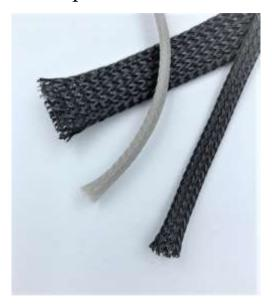
Polyester expandable sleeving is a flame-retardant sleeving with UL94 V-0 certified raw materials. It offers durable abrasion resistance in a wide range of industrial applications. The open weave construction allows an easy installation on a bundle of hoses and cables, even if some with bulky or large connectors. Totally expanded the sleeving can reach at least 1.5 times than the initial dimension.
